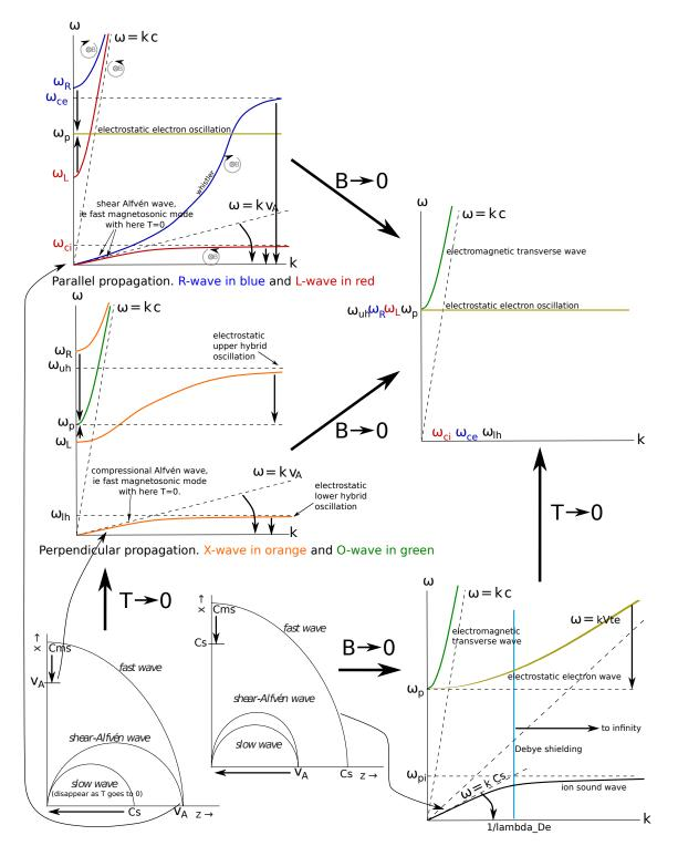
Figure 2: Different modes propagating in a homogeneous plasma. The black arrows show how the modes evolve when the temperature T or the background magnetic field  $B_0$  goes to zero. For example, to go from the lower-right to the upper-right diagram, one has to make  $T \to 0$ . The modes of the lower-right diagram then evolve according to the black arrows of this diagram, which act to transform it into the upper-right diagram. In the MHD part, the magnetic field is directed along z.
