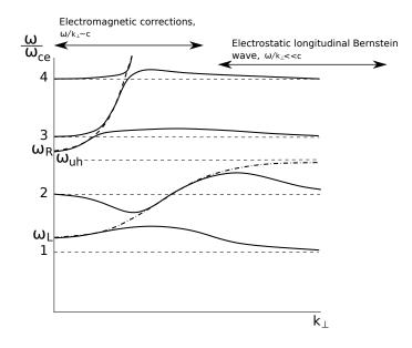
Figure 1: Full line: Dispersion relation of electron Bernstein waves, when the coupling with the X-mode at small k is taken into account. From Fitzpatrick (2011). The relative position of  $\omega_L$ ,  $\omega_{uh}$ ,  $\omega_R$  with respect to the cyclotron harmonics is not always as such, and depends on  $\omega_{ce}/\omega_{pe}$ . Dashed line: X-mode of the cold plasma.
