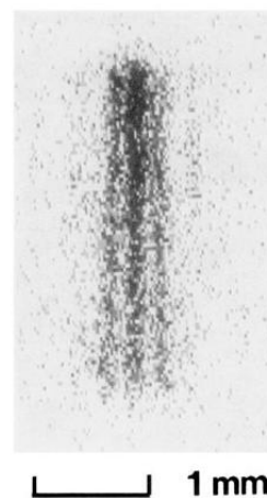
FIG. 2. The interference fringe pattern on the MCP for atoms with the initial velocity of approximately zero. The vertical length of the slit image is 2.8 mm. The spatial resolution of the picture is 20 and 32 \mu\text{m} for the horizontal and vertical directions, respectively. The narrowing of the fringe separation on the upper part is due to the damage of the double-slit structure. This figure contains approximately 6 \times 10^3 atomic counts.
